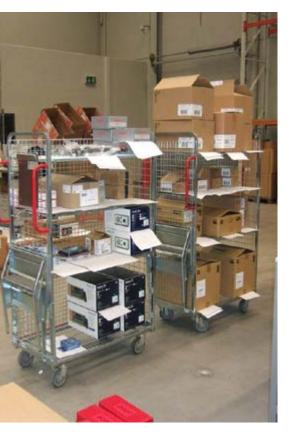
To combine the items from the four warehouse areas quickly and reliably to form orders, Duttenhofer uses a two-stage picking system consisting of so-called pallet and piece-picking. In the first stage, known as pallet-picking, various items for a number of different orders are taken from the pallet store, for example, and stored temporarily on an empty pallet at a central location.
